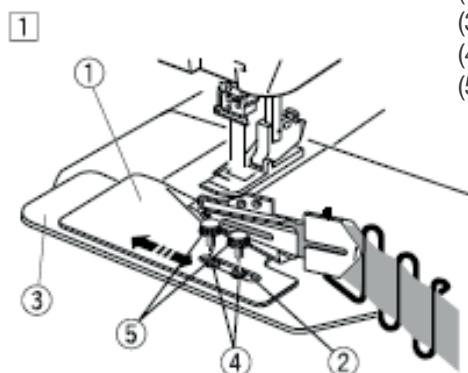
2. Align the folded tape and the needles by sliding the binder to the left or right. Tighten the two thumbscrews securely.
