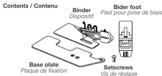
This binder is suitable for encasing a raw edge of a stretch fabric with a tape.
